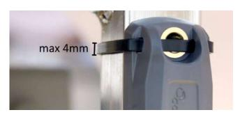
Polarization of Confidex Survivor™ is according to its longest dimension. This should be taken into account when using linearly polarized reader antennas.
